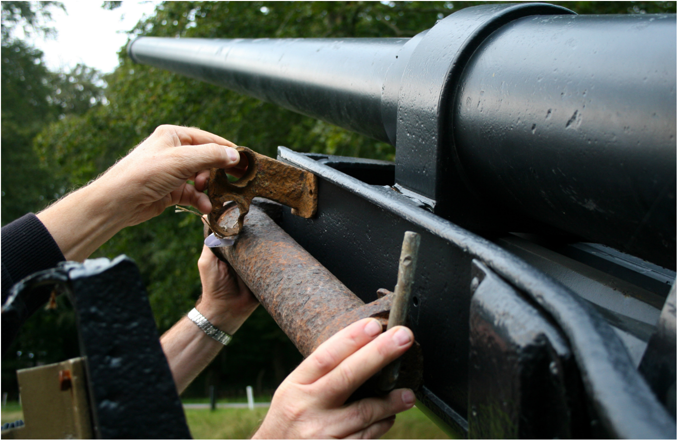
Figure 11. Refitting of the finds on the still existing gun 'Emil' (here in restored condition), with the help of Vincent Evers and Robert Markus of Museum Deelen. The brass part at the right is clearly bent by the explosion causing these parts to fall off. The 7.5 cm Flak M36 (f) of the 1./594 saw its last action in the Flak-Stellung in Meinerswijk, Arnhem, and was recovered there in 1996 (photo: Author, August 2023).
