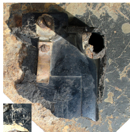
Figure 14. Detail of the bakelite interior with diagram and the BAL stamp (photo: Author).
