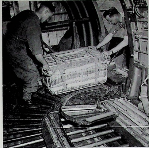
Men of the Royal Army Service Corps load a supply pannier into a Dakota. A roller track is visible in the foreground over which the panniers could be slid. This simplified and speeded up the loading and ejection of supplies by the Air Despatchers. The photograph comes from Frank Steer's book 'Arnhem, The Fight to Sustain'. (Courtesy Imperial War Museum, London, CH 12945)
