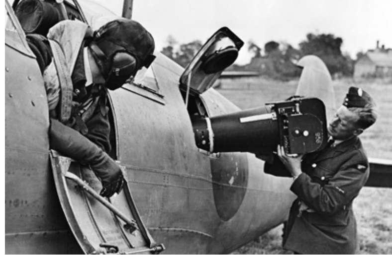
▲ An aerial camera being loaded into a vertical position in a Spitfire at RAF Benson
