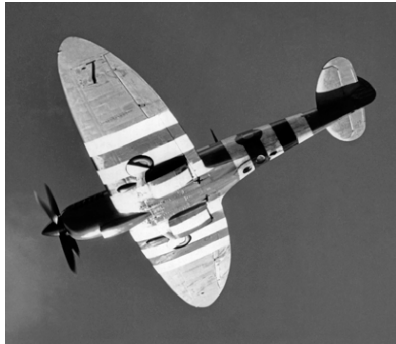
▲ A 541 Squadron Spitfire XI showing the rear-mounted under-side cameras used for taking high-level vertical images
